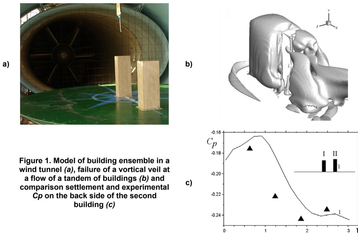
**Figure 1. Model of building ensemble in a wind tunnel (a), failure of a vortical veil at a flow of a tandem of buildings (b) and comparison settlement and experimental  $C_p$  on the back side of the second building (c)**
