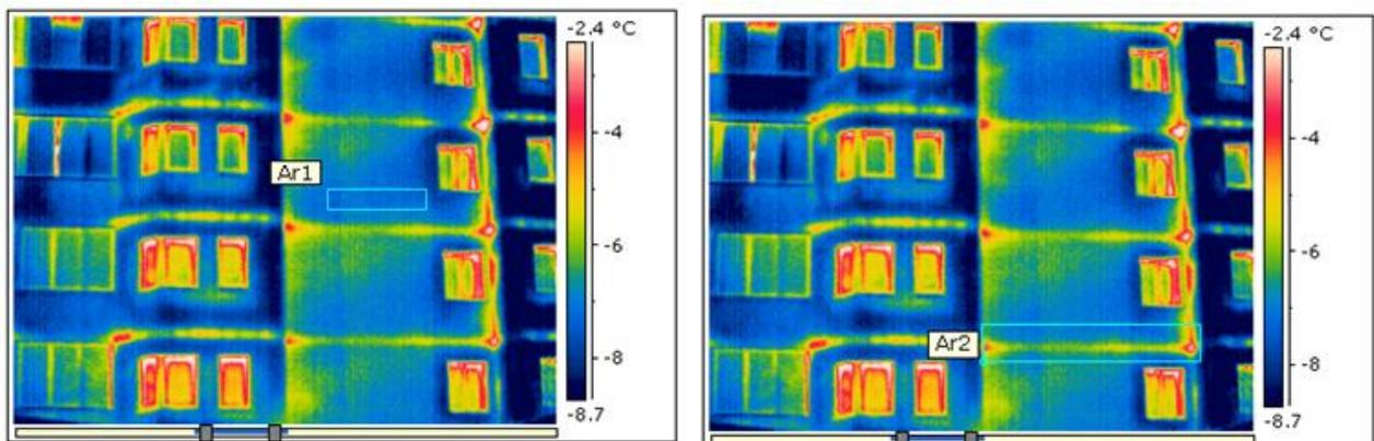
Figure 1. Results of processing data from thermograms of a panel building, obtained under field conditions
