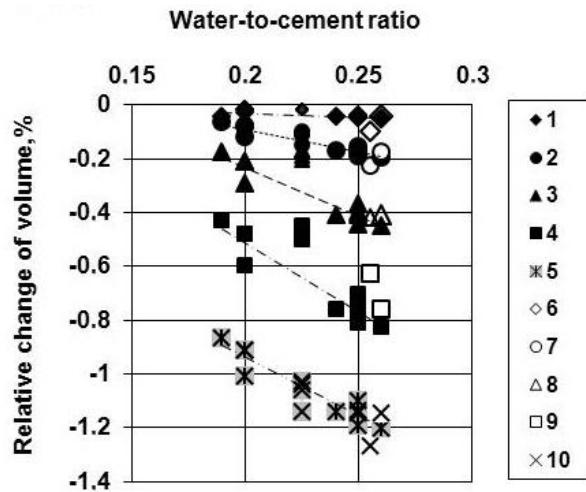
**Figure 6. Water-to-cement ratio dependence of radiation-change of volume of Portland cement stones with and without various superplasticizers additives – after radiation treatment with different fluency of fast neutrons charged above 0.8 MeV**
