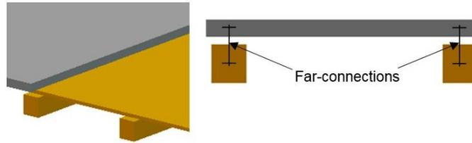
Figure 4. Part of the 3D FE model of the composite ceiling
