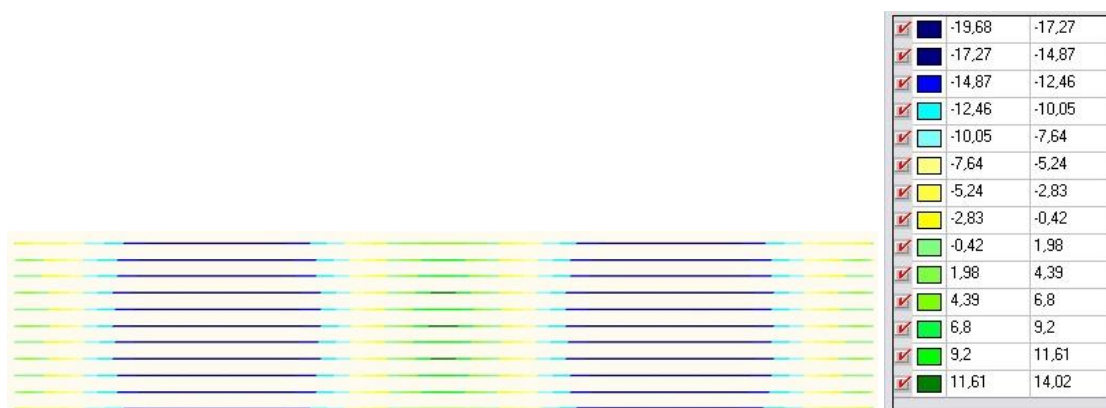
Figure 9. Top reinforcement bar axial force isofields (daN)
