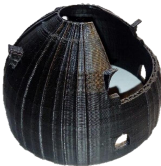
Figure 1. Dome house model printed on a 3D printer
