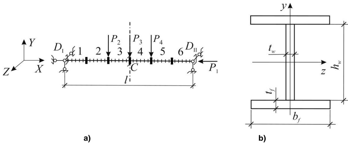
Figure 3. Bar system with two supports: a – design diagram applying the basic geometry of the object with subdivision on finite elements: 1–6 – bar numbers, b – bar cross-section in local system of axes
