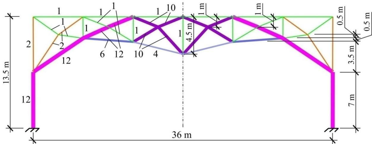
Figure 6. Result of frame optimization
