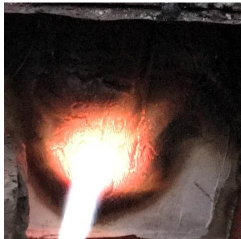
Figure 2. Exposure to flame in the test installation
