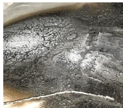
Figure 4. The state of the silica/glass fiber from the heated side (about 1200 °C) after the tests
