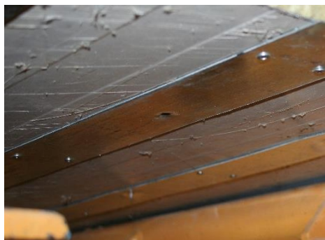
Figure 14 and 15. Process of pulling out a screw (left), hole in the plate after the pull out (right)
