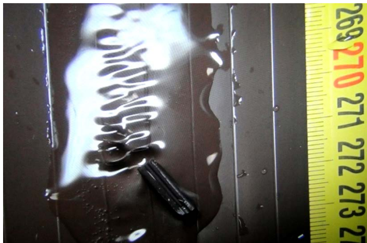
Figure 3. Single obstacle in the form of a rectangular bar with displacement
