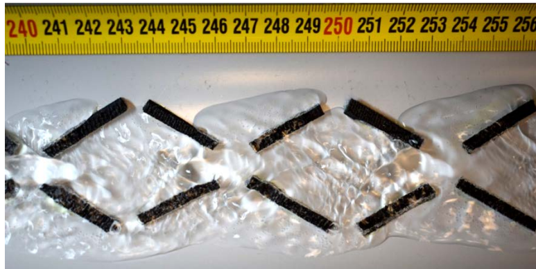
Figure 5 Grouped obstacles in the form of bars of rectangular cross-section, located at an angle of 120 degrees
