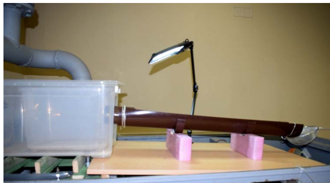
Figure 1 Side view of a special stand in the form of an open inclined chute of 130 mm diameter for performing experiments
