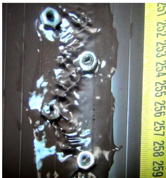
Figure 4. Grouped obstacles in the form of identical polyhedral figures displaced from the axis of the chute
