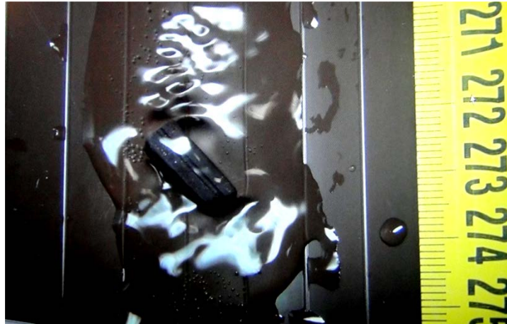
Figure 2. A single obstacle in the form of a rectangular bar (with a measuring ruler on the right)
