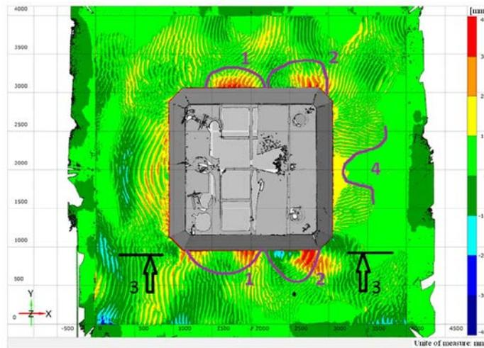
**Figure 6. Bottom profile near the Platform model after experiment No. 5:**
