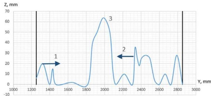
**Figure 14. Interference (3) during the movement of sand waves (1, 2) along the rear edge of the Platform as a result of the experiment No. 4 (Cross-section 1-1 in Figure 5)**
