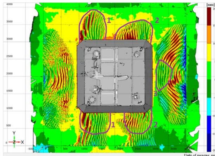
**Figure 2. Bottom profile near the Platform model after experiment No. 1:**
