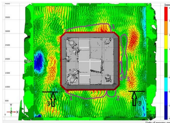
**Figure 3. Bottom profile near the Platform model after experiment No. 2:**
