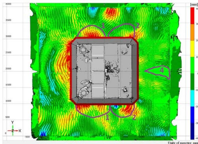
**Figure 7. Bottom profile near the Platform model after experiment No. 6:**
