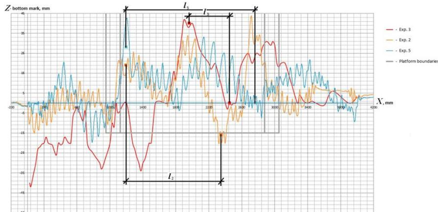
**Figure 8. The profiles of the bottom surface along the left side of the Platform in the cross-section 3-3 along the side of the Platform model as a result of experiments NoNo. 2, 3 and 5**
