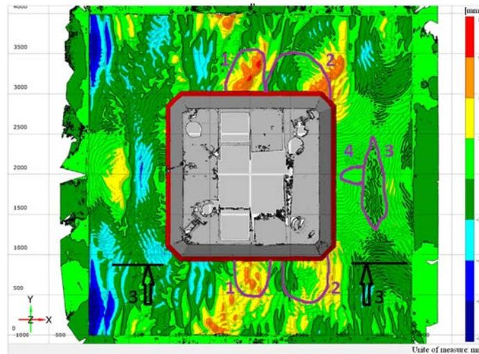
**Figure 5. Bottom profile near the Platform model with a protective skirt with a length of penetration into the soil  $H = 0.20$  m after experiment No. 4:**
