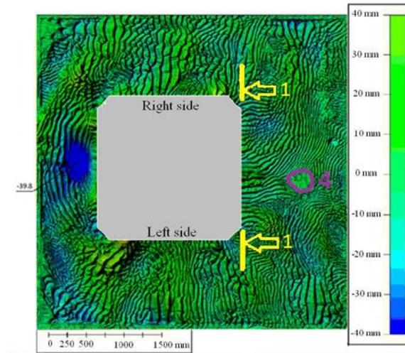
**Figure 4. Bottom profile near the Platform model after experiment No. 3:**
