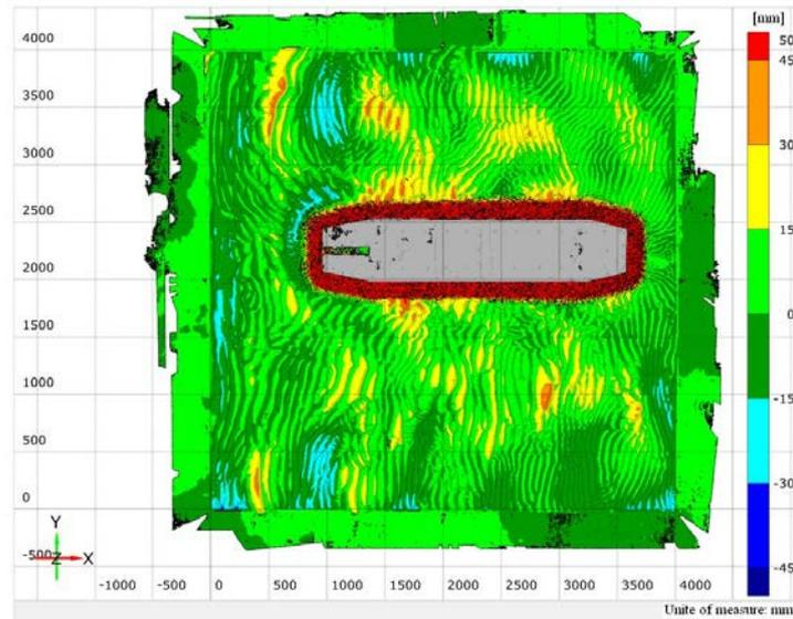
**Figure 12. Bottom profile near the Barge model with protective underwater riprap prism after experiment No. 10**
