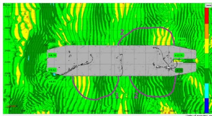
**Figure 9. Bottom profile near the Barge model after experiment No. 7:**
