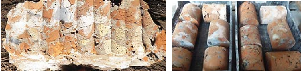
Figure 4. The structure of the brick aggregate concrete vaults and core samples in the compressive test
