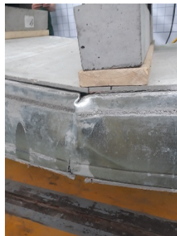
Figure 9. The destruction in the "dangerous" section
