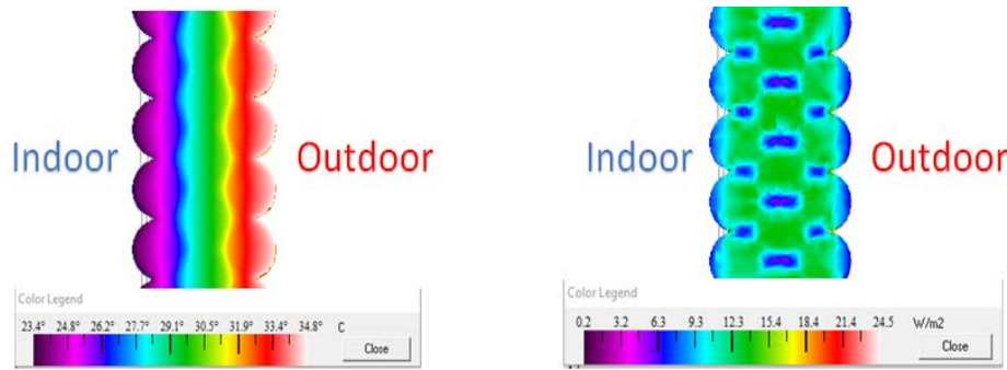
Figure 12. Temperature Gradient (OC) and Heat Flux Gradient (W/m 2 ) for Triple-Layer Bamboo Wall
