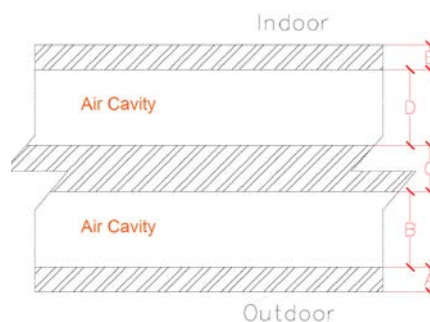
Figure 5. Wall Equivalent for 2 layers bamboo wall. A, C and E is a hypothetical solid material with the same thermal properties as the Bamboo-Moso and B and D are air cavities
