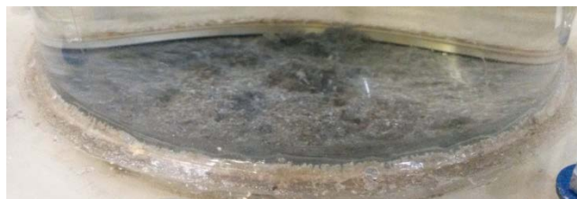
Figure 11. Mesh with a cell of 1.0 mm with 100% of debris without paint plates, borated water
