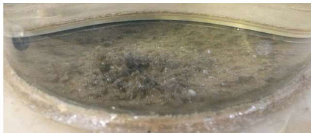
Figure 10. Mesh with a cell of 1.0 mm with 60% of debris without paint plates, borated water
