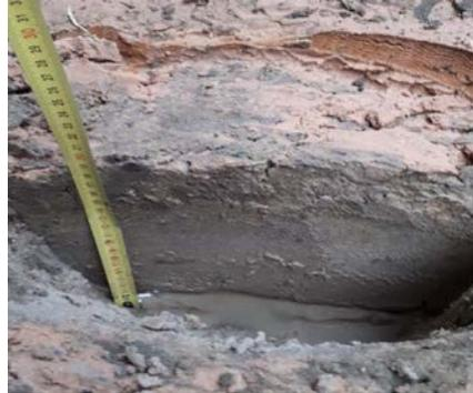
Figure 5. The groundwater level during the excavation process at a depth of (1.9 m)
