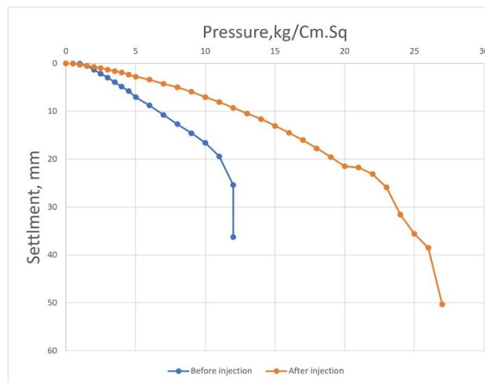
**Figure 17. The results of load-settlement in points (2, 4) at a depth of (1.1,1.2 m) respectively before and after the injection of the resin**
