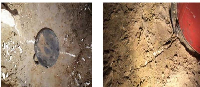
**(A) The location of the steel plate. (B) The soil-resin under the load.****Figure 8. The steel plate as placed in-situ in point number (5). (A) The setting up the plate on the resin-soil composition, (B) The soil-resin under the load in this point**
