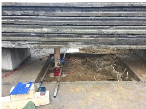
**Figure 9. The plate load test under the load in point (3)**
