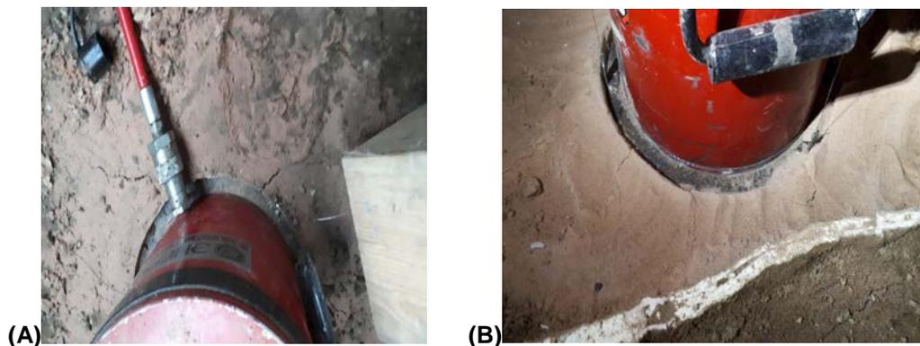
Figure 15. The soil under the ultimate load and cracks shown as a sign of the soil failure. (A) failure in the reference, (B) failure in the injected plot
