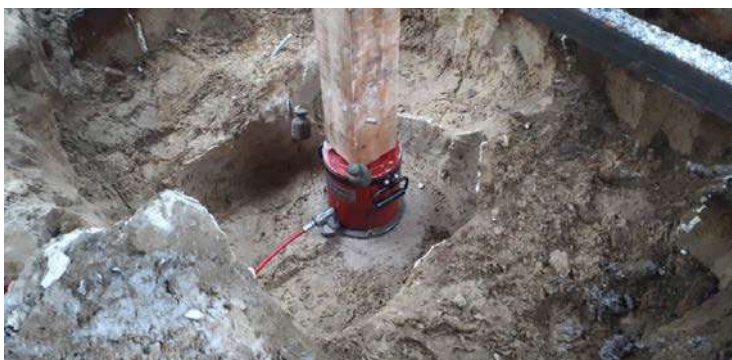
Figure 10. The plate load test under the load in point (4)
