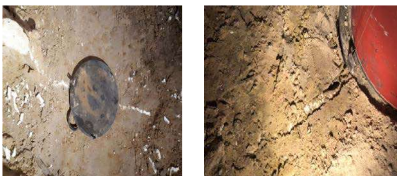
(A) The location of the steel plate. (B) The soil-resin under the load.
