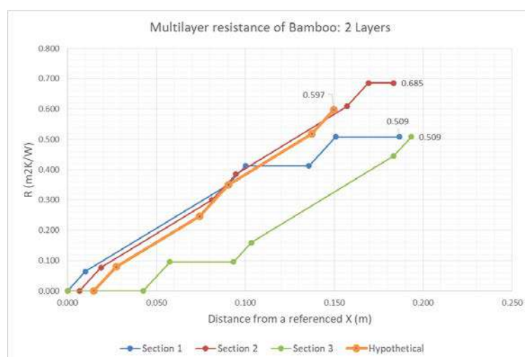
Figure 7. Thermal resistance in the axis 1, 2 and 3 and an equivalent wall, from a referenced x
