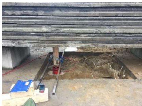
Figure 9. The plate load test under the load in point (3)
