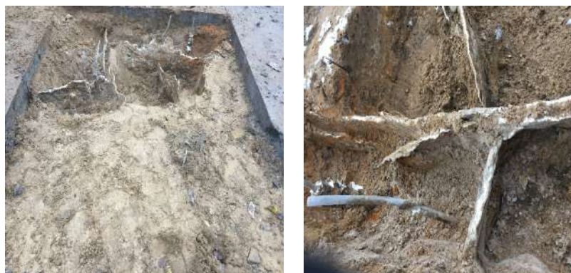
Figure 13. Different sections of the resin injection in the injected plot at depth (0.4 m).
