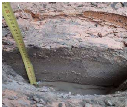
Figure 5. The groundwater level during the excavation process at a depth of (1.9 m)
