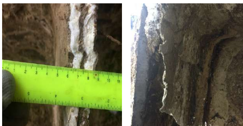
Figures 14. Different sections of the resin diffusion in the injected plot at depth (1.1 m)
