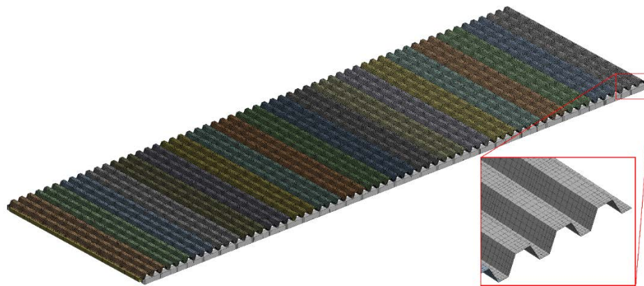
Figure 4. A FE-model of a corrugated sheet panel with accurate geometry modelling. Typical model 20m* 6m contains ca. 4 million degrees of freedom. Each sheet is highlighted by different colors.
