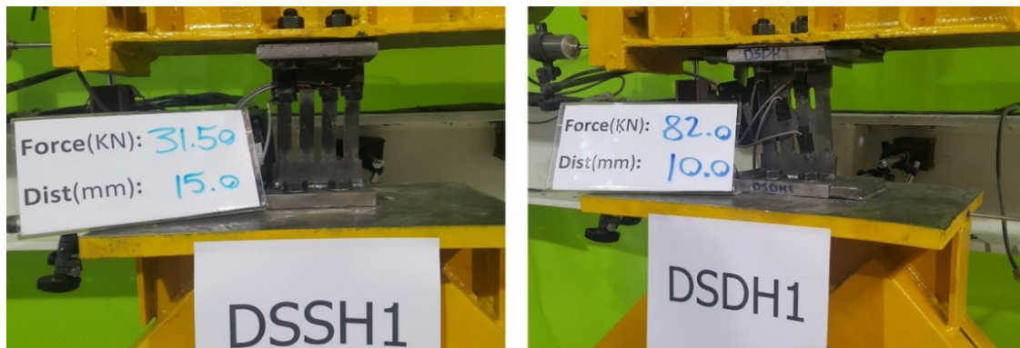
Figure 13. The deformation of DSSH1 and DSDH1 at maximum force.
