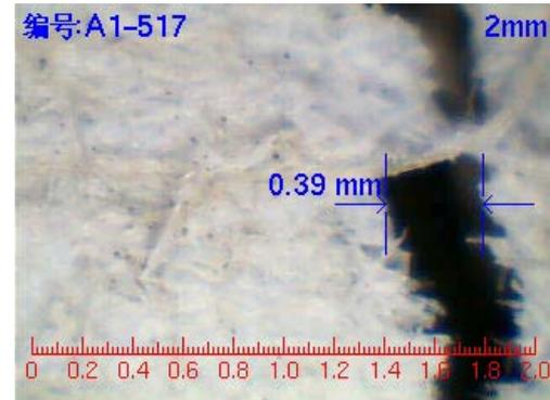
Figure 2. Crack width observation reading viewport.
