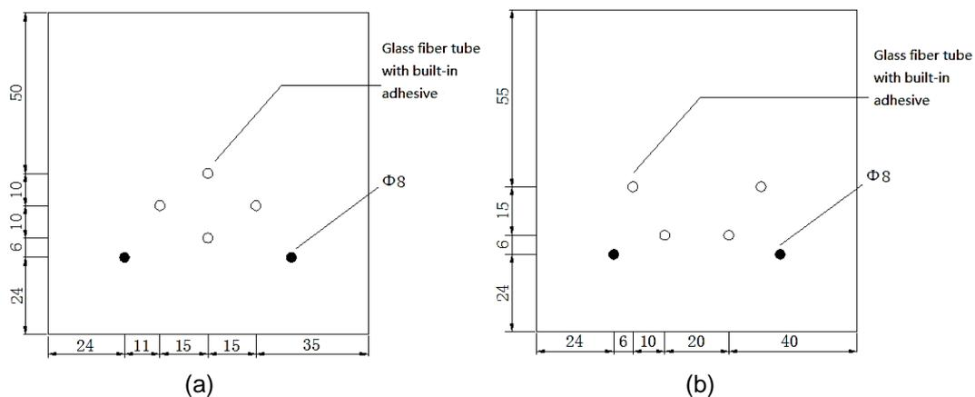
Figure 3. How to place the glass fiber tube in the test piece:(a) the glass tube is placed in a diamond shape (b) the glass tube is placed in an inverted trapezoid.
