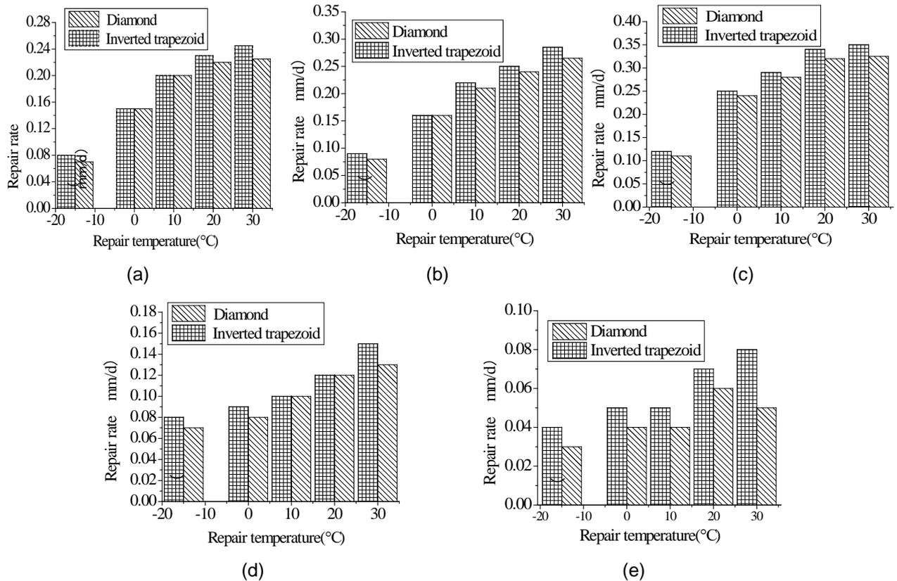
**Figure 12. Change in repair rate as the fiberglass tube is placed: a) Initial crack width is 0.4mm; b) Initial crack width is 0.6mm; c) Initial crack width is 1.0 mm; d) Initial crack width is 1.5 mm; e) Initial crack width is 2.0mm.**
