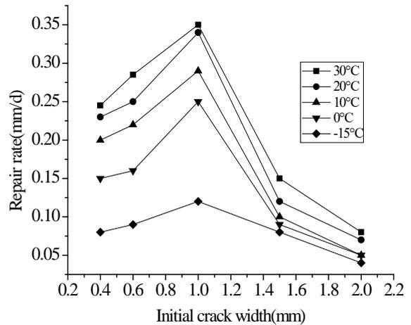
**Figure 11. Repair rate as a function of initial crack width (inverted trapezoid).**
