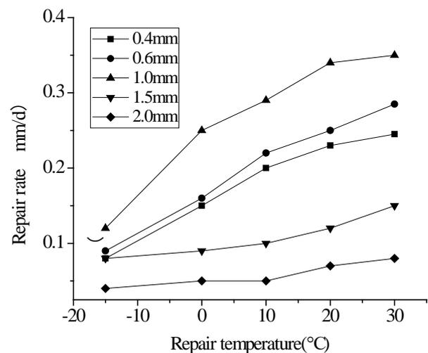
Figure 9. The change of repair rate with temperature when the glass fiber tube is placed in inverted trapezoid.
