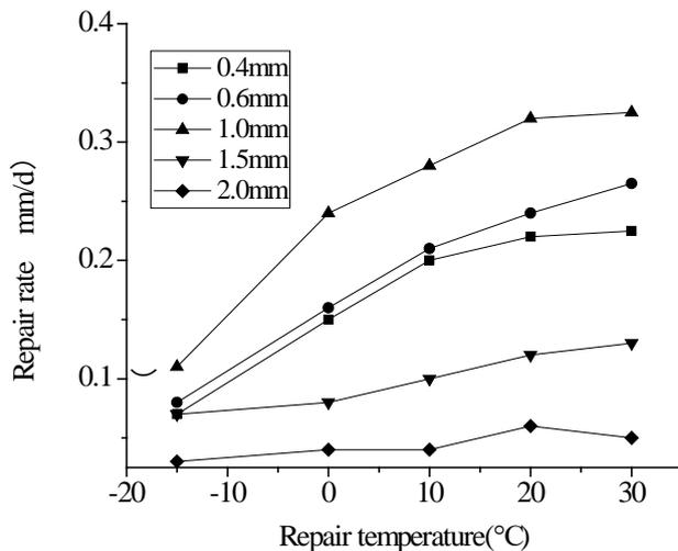
Figure 8. Change of repair rate with temperature when the glass fiber tube is placed in a diamond shape.
