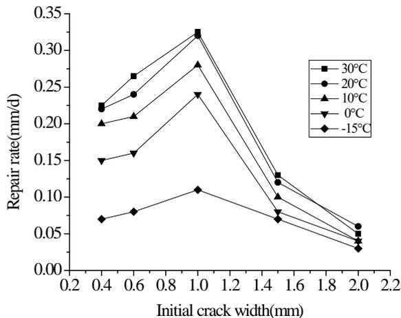
**Figure 10. Repair rate as a function of initial crack width (diamond).**
