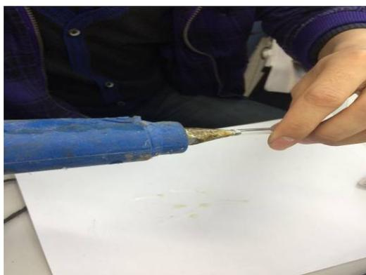
**Figure 4. GLUE GUN GT-10 hot melt glue gun.**
