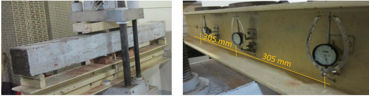
Figure 4. Beam test setup (left) and position of the dial gauges placed at steel loading frame (right).
