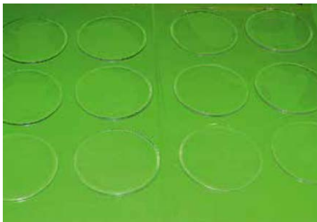
Figure 1. Silicone film of a thickness of 1 mm [21].
