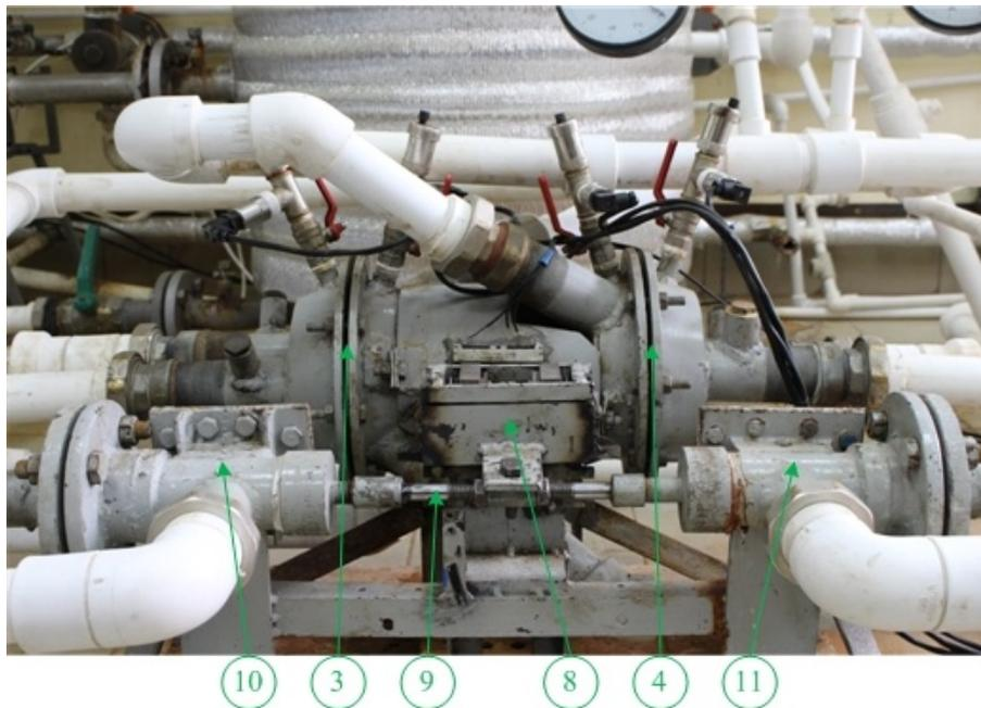
**Figure 2. Physical form of experimental unit of IHP on the basis of double-flow membrane pump: 3 – Membrane pump left section; 4 – Membrane pump right section; 8 – Switching shock valves mechanism; 9 – Link rod; 10 – Left shock valve; 11 – Right shock valve.**
