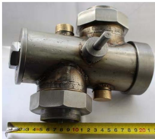
**Figure 3. Pulsed flow distributor.**
