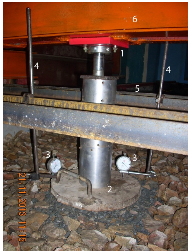
Figure 6. Photograph of large-scale model experiment set-up: 1 – hydraulic cylinder of jack, 2 – rigid stamp, 3 – dial indicators with a scale, 4 – indicator mounting rods, 5 – bench mark beams, 6 – traverse.
