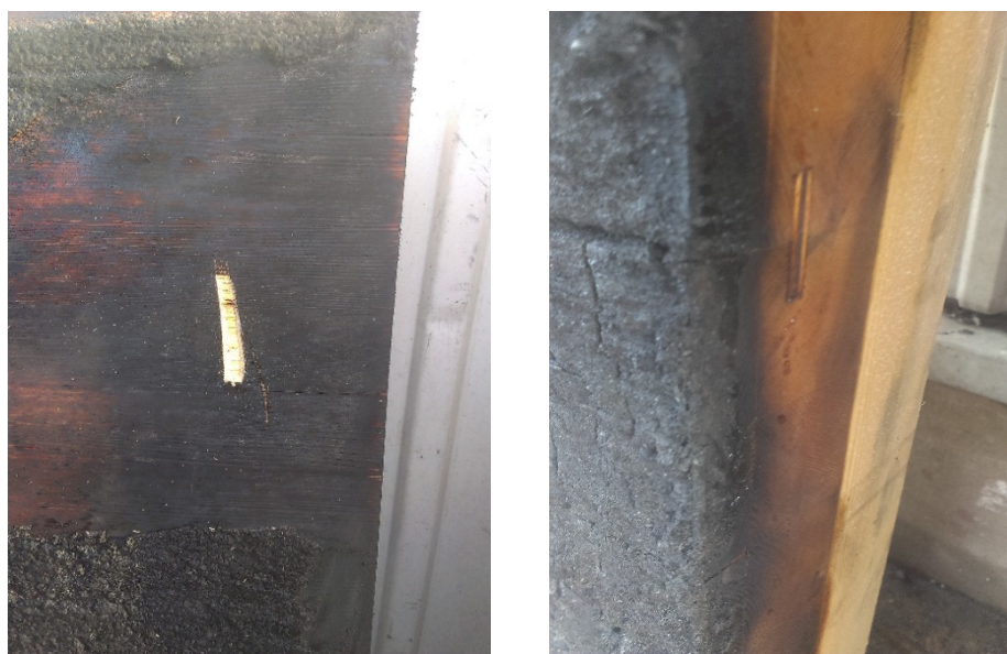
Figure 7. Development of foamed coil after the testing of sample 7.
