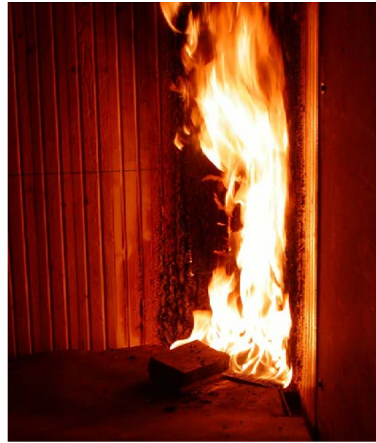
Figure 6. Sample 4 – bloating of the lacquer.
