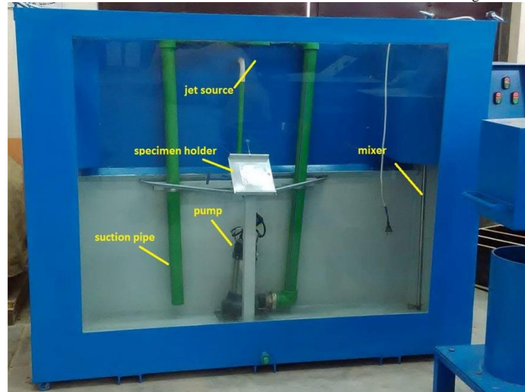
Figure 1. The used water-jet abrasion testing apparatus.
