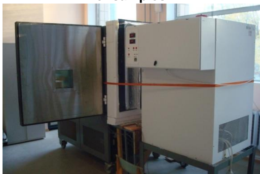
Figure 3. Testing a masonry fragment in the climate chamber.
