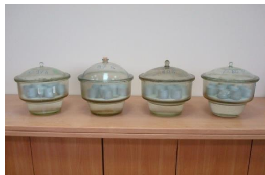
Figure 2. The excitatory method for determining the sorption moisture of samples.
