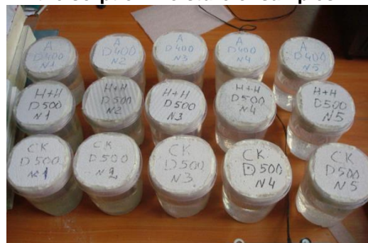
Figure 4. Determination of vapor permeability of samples.
