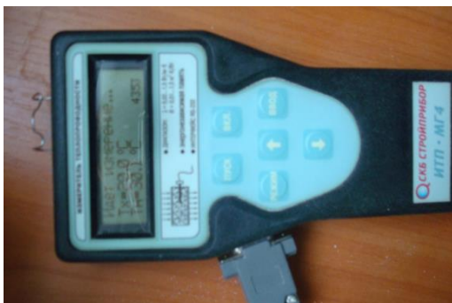
Figure 1. Measurement of thermal conductivity of samples.
