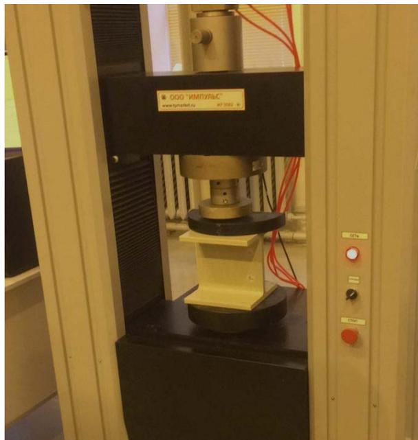
**Figure 7. Test of the web of the I-beam under the local compressive load.**
