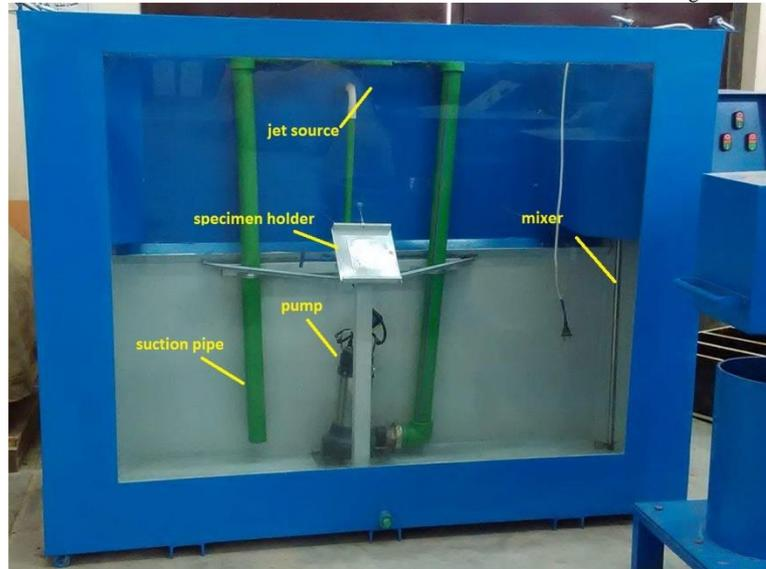
Figure 1. The used water-jet abrasion testing apparatus.
