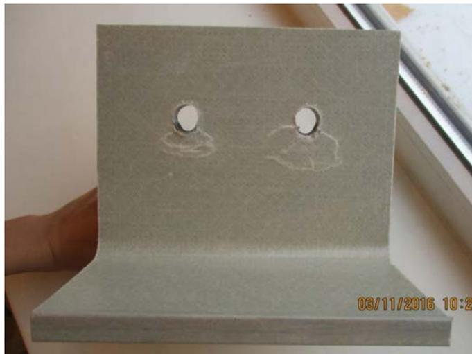
**Figure 12. Failure of joints under the compressing load in case of load applied perpendicular to the direction of pultrusion.**
