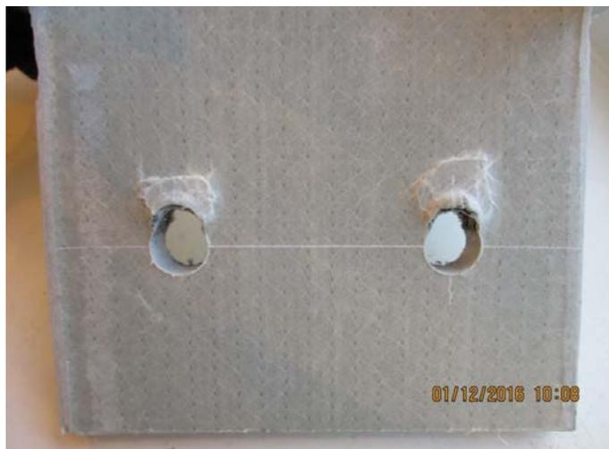
**Figure 13. Failure of joints under the compressing load in case of load applied parallel to the direction of pultrusion.**
