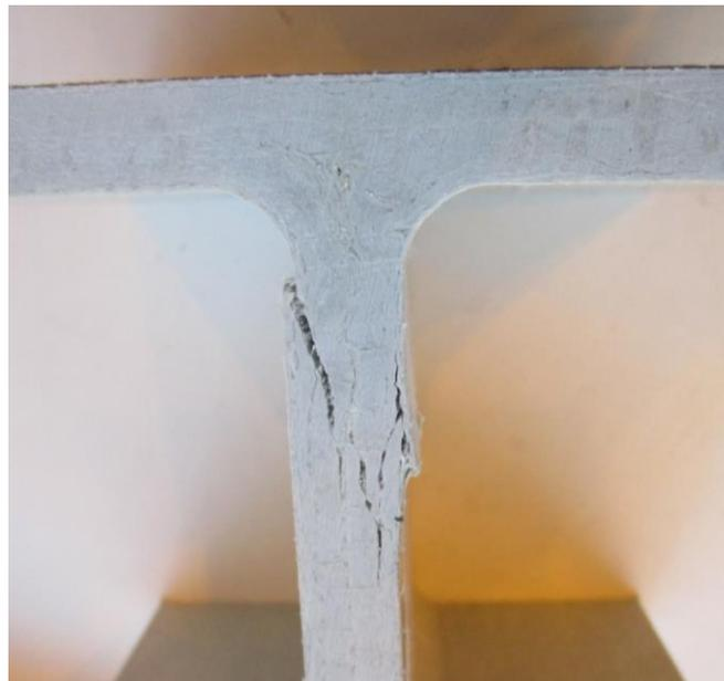
**Figure 15. Failure of the web of the I-beam under the ultimate local compressive load.**
