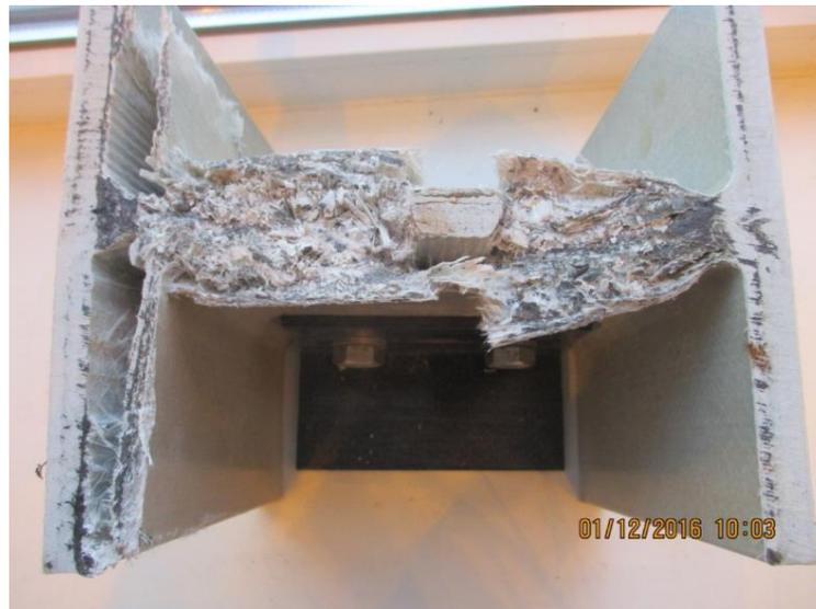
Figure 17. Failure mode of the I-beam under the crumbling load.
