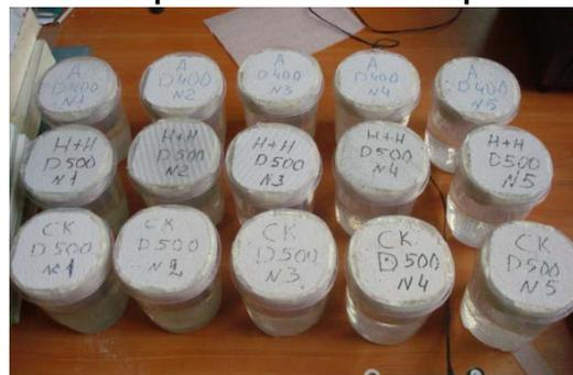
Figure 4. Determination of vapor permeability of samples.
