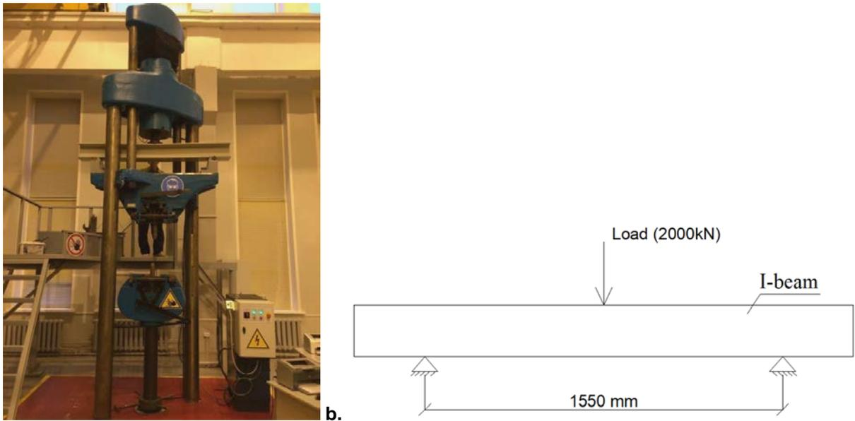
Figure 4. Flexural bending test of I-beam from PFRP: a –hydraulic press; b – scheme of a loading.
