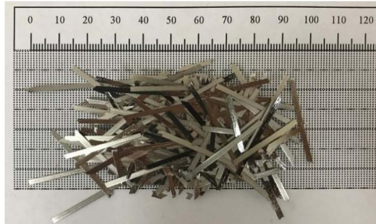
**Figure 6. Amorphous fiber (Fe-B-C system).**
