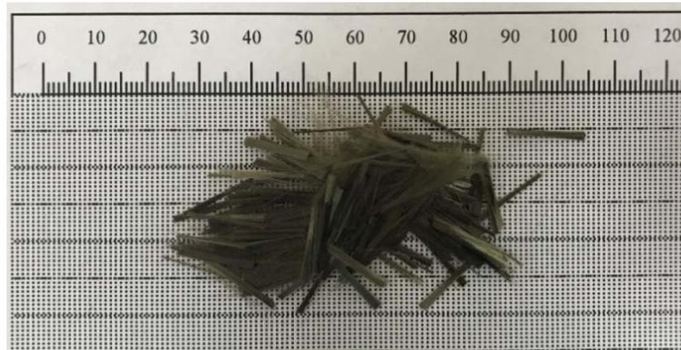
**Figure 2. Basalt fiber.**
