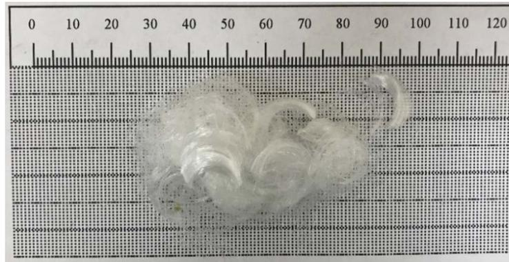
**Figure 1. Polypropylene fiber.**
