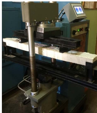
Figure 6. Load application to the sample according to the diagram (Figure 2).
