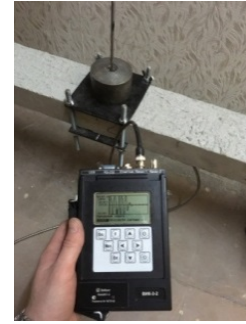
Figure 5. Excitation of the first forms of the sample oscillation with the determination of its natural frequencies.
