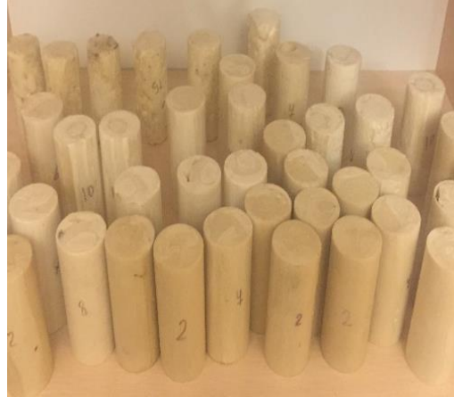
Figure 4. The prepared resin's samples of different densities.
