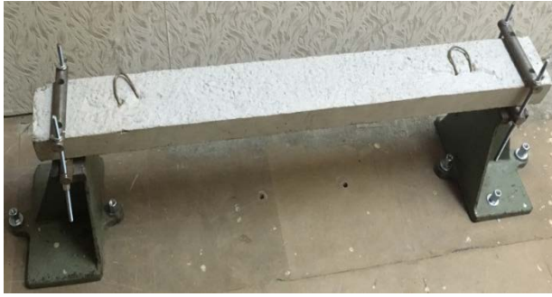
Figure 4. Fixing the test sample on the stand.
