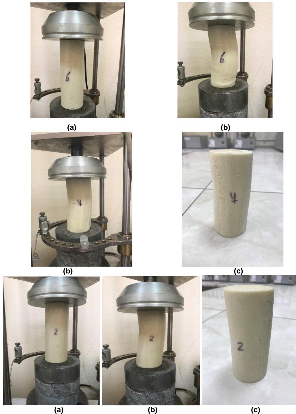
Figure 6. Some of the resin samples during the uniaxial compression tests. (a) The sample during the compression test; (b) The sample at the end of the compression process; (c) The sample after the release of the uniaxial forces
