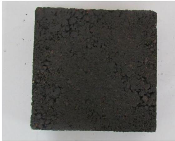
**Figure 3. The asphalt concrete sample in the shape of square slab (300×300×100mm).**
