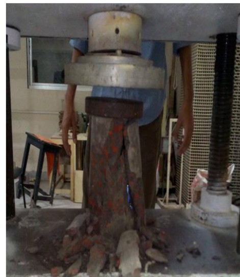
Figure 6. Specimen fracture pattern after compressive strength test.
