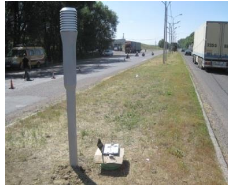
Figure 3. View of surface part of the temperature and moisture automatic measurement system on the highway ‘Almaty-Bishkek’.
