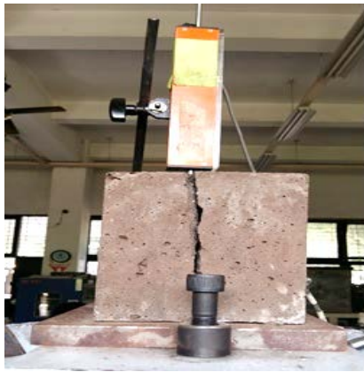
a. GPC specimen without PVA fibre
