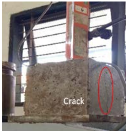
c. GPC specimen with 0.4% PVA fibre
