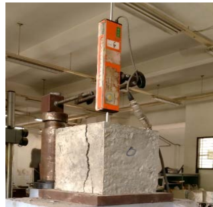
b. OPC specimen without PVA fibre
