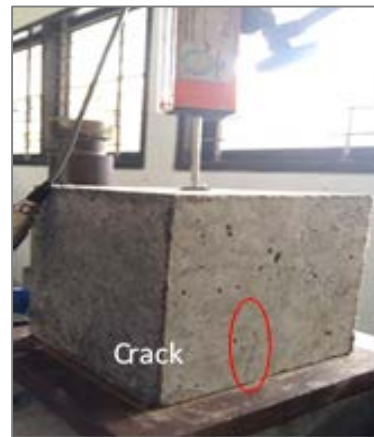
d. OPC specimen with 0.4% PVA fibre
