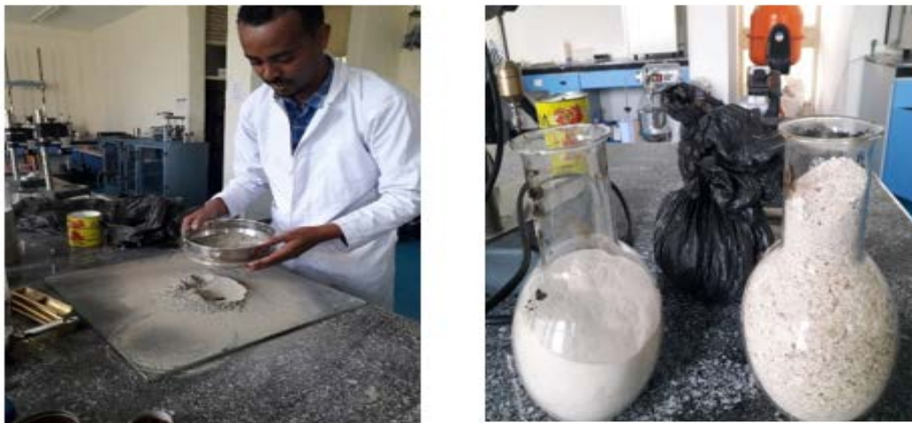
Figure 1. Sample preparation for Portland cement and Waste Animal Bone.
