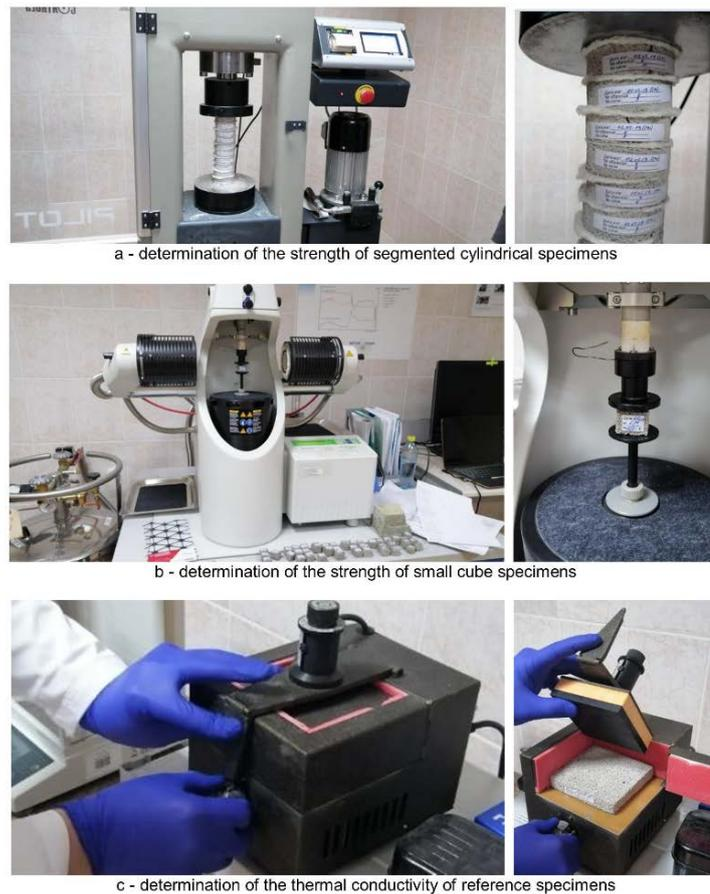
**Figure 3. Laboratory testing of foam concrete specimens.**
