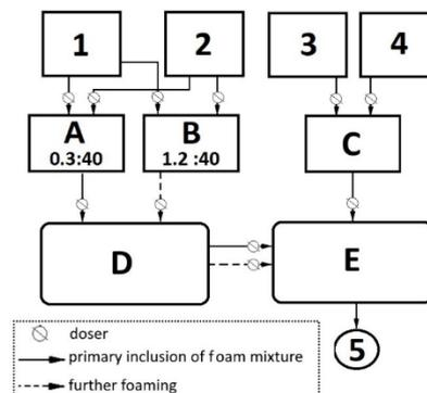
**Figure 1. The technology of foam concrete preparation by the method of TSF: 1 – water; 2 – foam concentrate; 3 – cement; 4 – sand; 5 – finished product; A – the container for the low-concentrated mixture of the plasticizing additive of a foam concentrate in water 0.3:40 l, B – the container for a mixture of the modified foam concentrate in water 1.2:40 l, C – the cement-sand mixer, D – the foam generator, E – the mortar mixer.**
