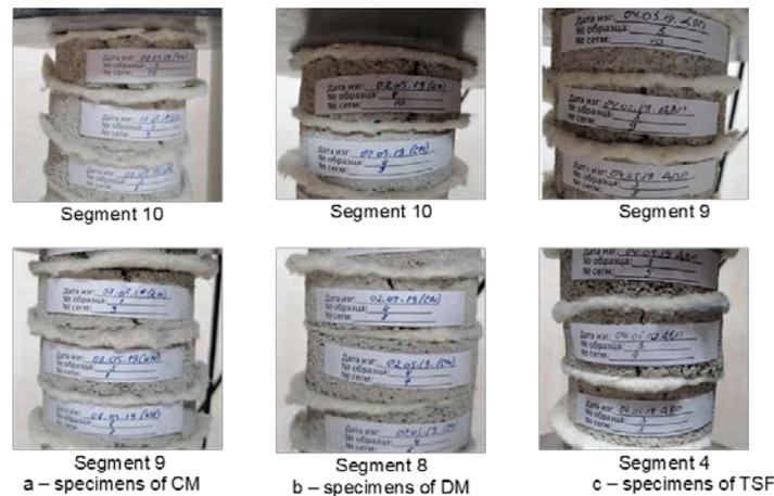
Figure 5. Weakest segments of specimens.
