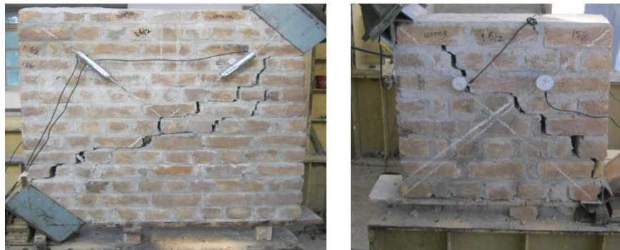
Figure 6. Typical damage pattern during diagonal tension tests.
