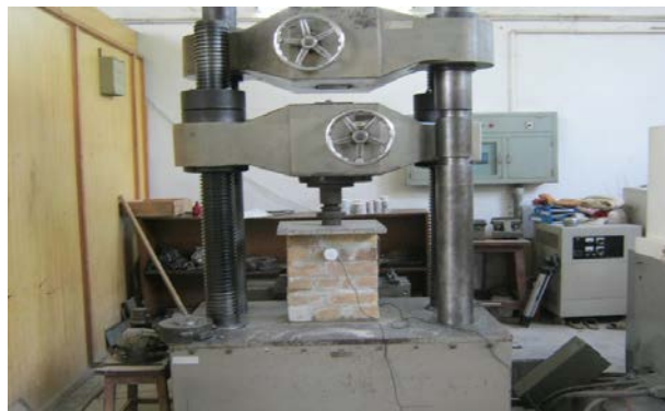
Figure 1. Test setup for compressive strength of masonry prisms.
