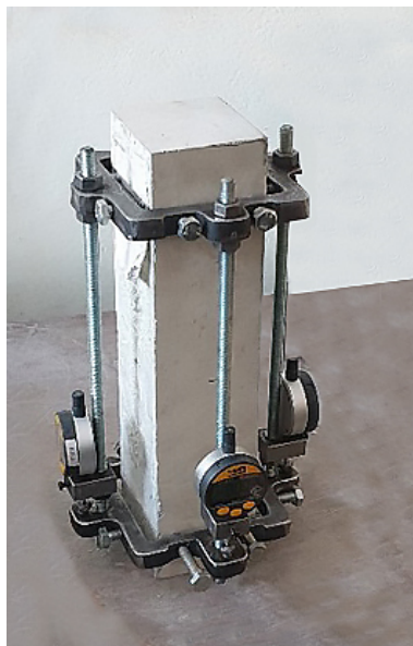
Figure 2. Concrete sample modulus of elasticity under compression testing.
