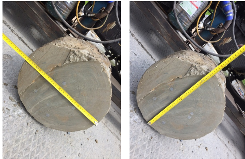
Figure 10. Diameter of drill-injection pile “N-1” after extraction.
