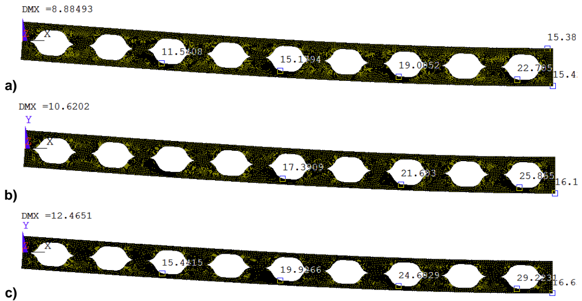
Figure 3. Stress state of simply supported beams l-h_w-1.2-19-1.78\text{cm}-\beta-1.5-0.75 with different opening height:
