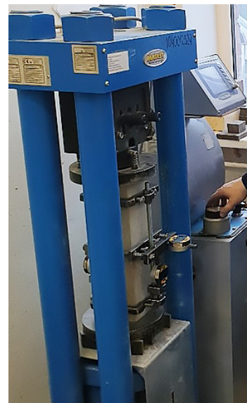
Figure 2. Concrete sample modulus of elasticity under compression testing.
