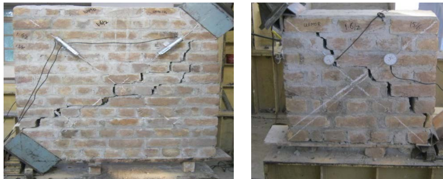
Figure 6. Typical damage pattern during diagonal tension tests.
