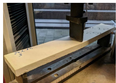
c) 3-point bending ultimate load determination
