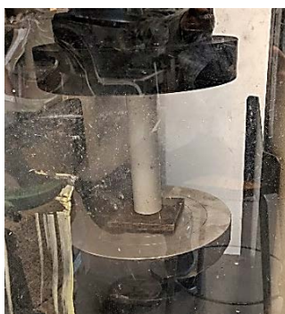
a) Compressive ultimate load determination
