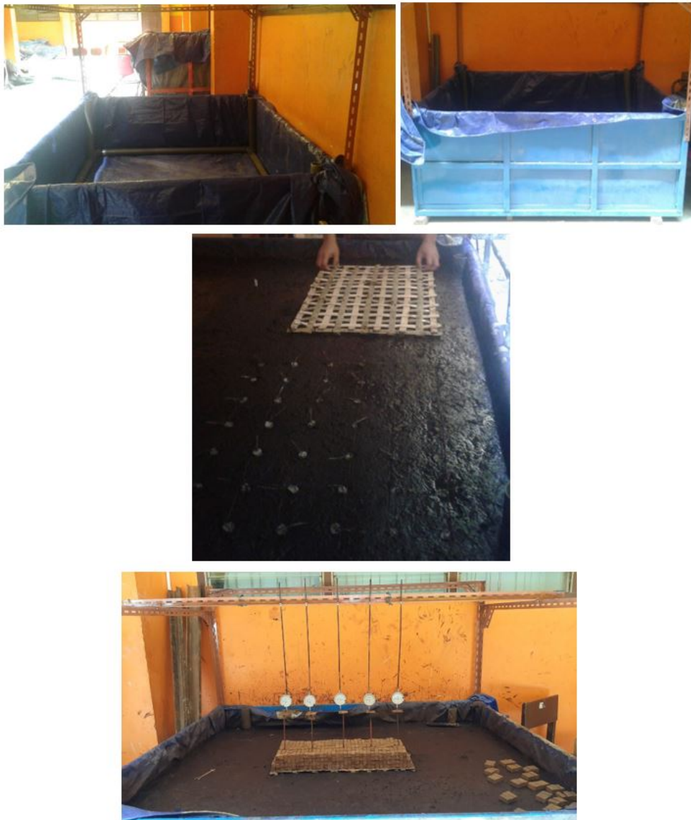
Figure 5. Photographs of embankment load test for box sized of 2 m x 1.5 m.
