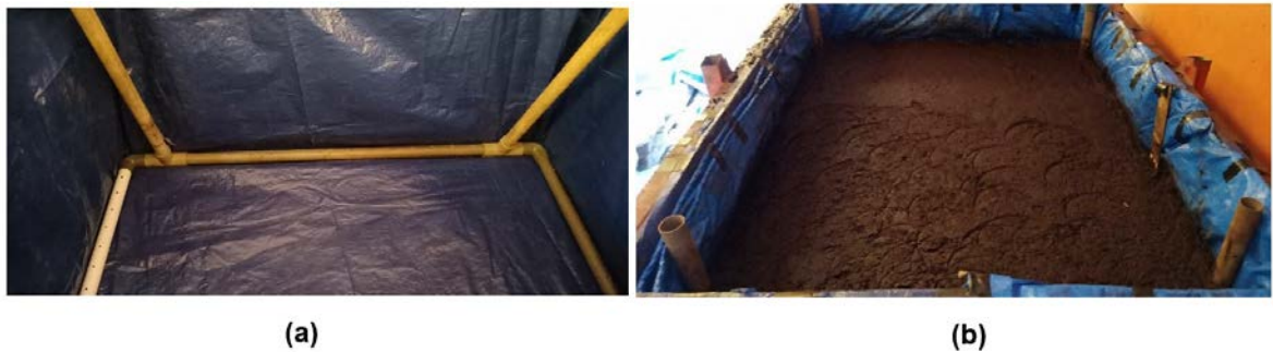
Figure 2. Photographs of (a). Test box with water drainage pipe; (b). Compacted peat soil.
