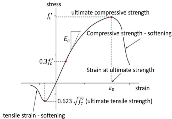
**Figure 3. Uniaxial stress-strain curve adopted for concrete.**
