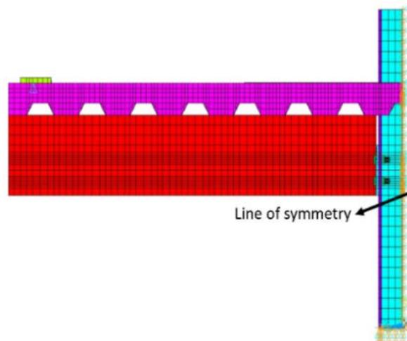
**Figure 2. Typical finite element model with Boundary conditions.**
