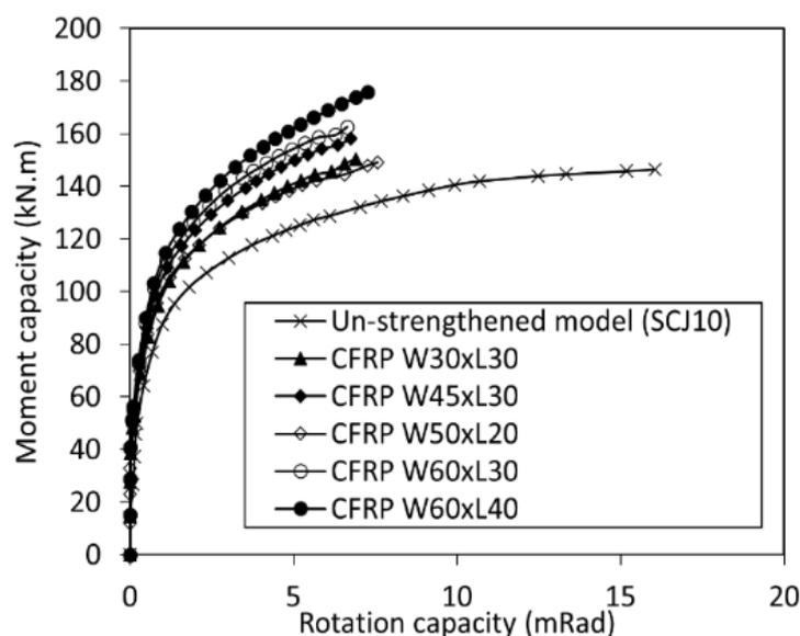
**Figure 8. Moment-rotation curves for un-strengthened and strengthened models.**
