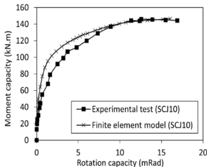
**Figure 5. Comparisons between experimental and FEM results.**
