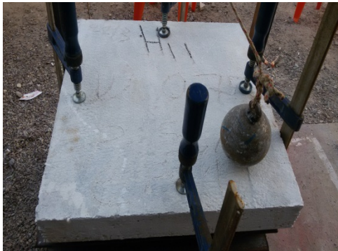
Figure 5. Failure of composite slabs under Impact force.
