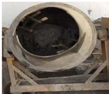
Mixing concrete by tilting drum mixer
