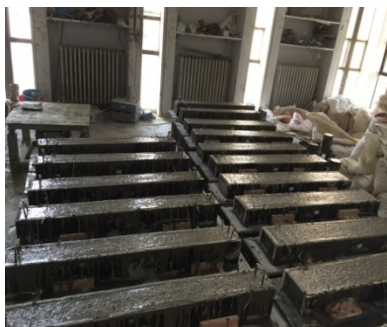
Casting concrete into molds
