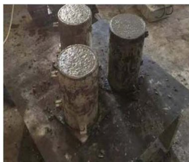
Casting concrete into cylinders
