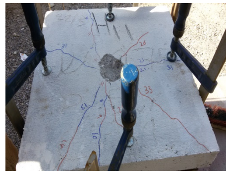
Figure 5. Failure of composite slabs under Impact force.
