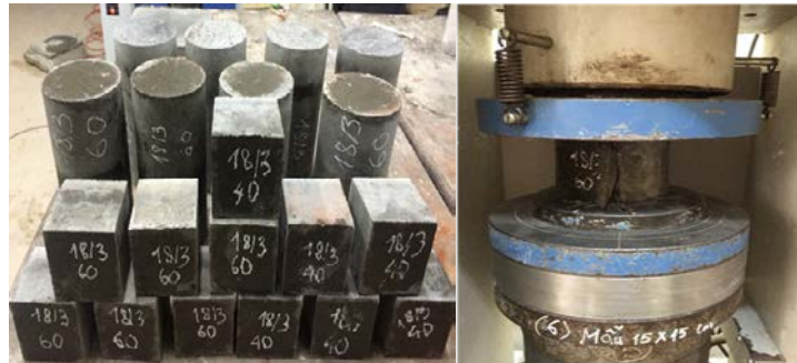
Figure 5. Preparation of specimen and compression test.
