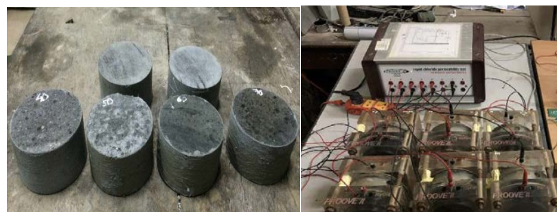
Fig. 7. Preparation and example of a chloride penetration test
