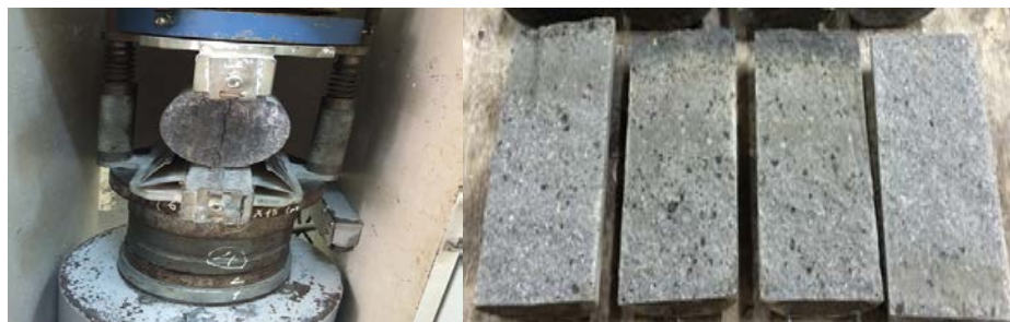
Figure 6. Example of the splitting tensile strength test.
