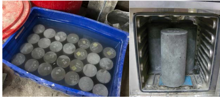
Figure 8. Soaking and drying concrete samples.
