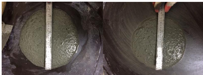
Figure 4. Example of measuring the slump flow of fine-grained concrete.
