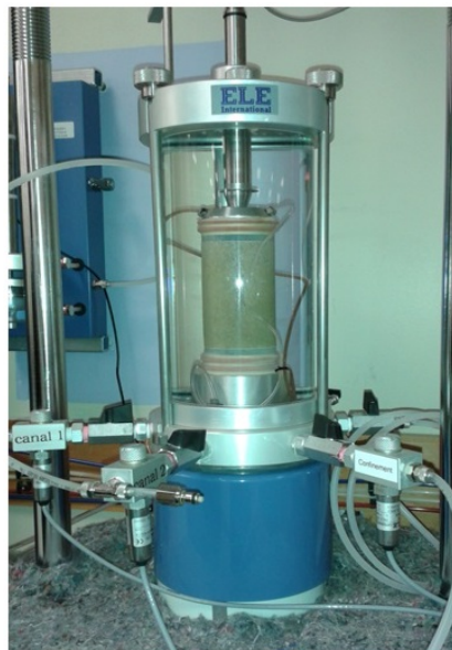
Figure 8. The triaxial cell.
