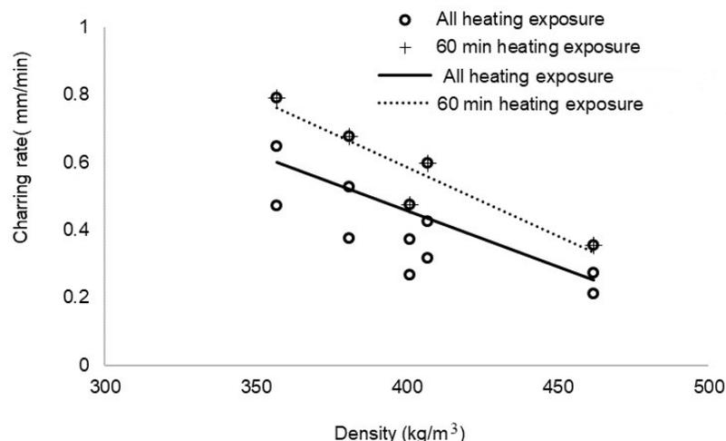
**Figure 7. Relationship between density and charring rate.**
