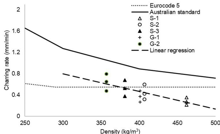
Figure 8. Comparison charring rate with other standard.
