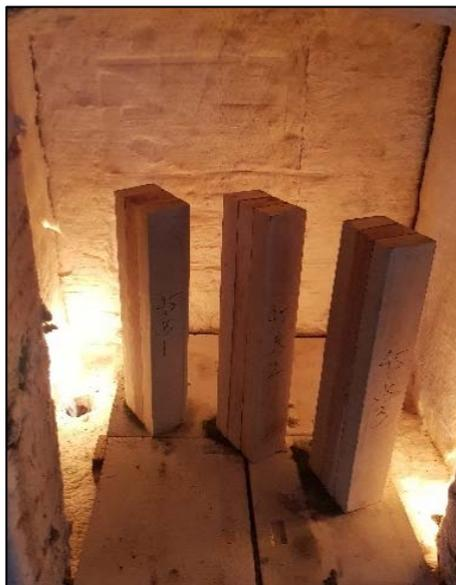
**Figure 3. Fire test set up.**
