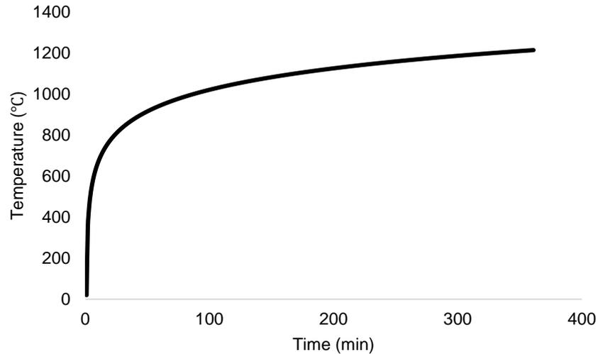
**Figure 2. Temperature growth curve according to ISO 834 [14].**
