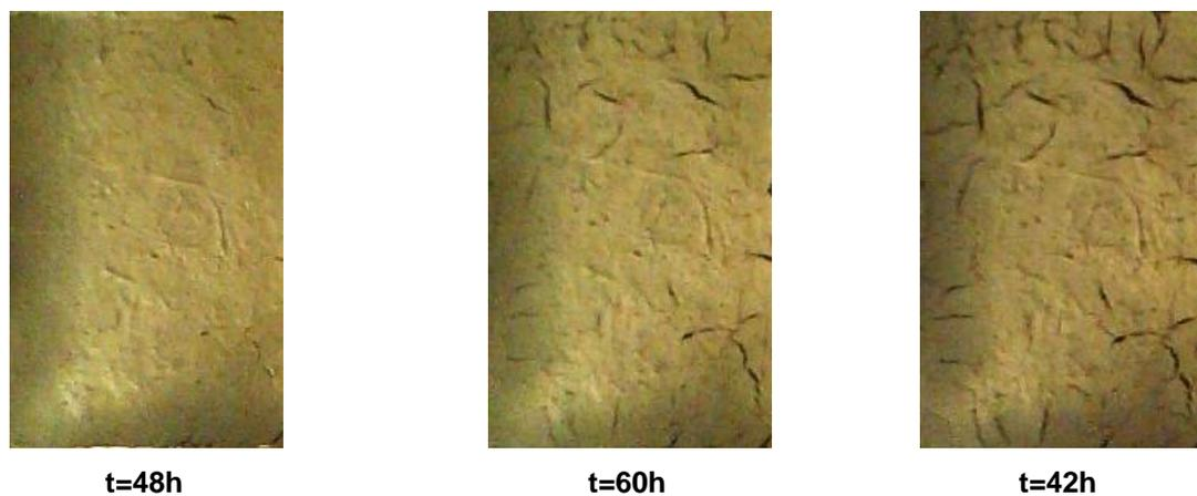
Figure 10.c cracks pattern evolution by drying (reinforced specimen  $\eta_f = 0.5\%$ )
