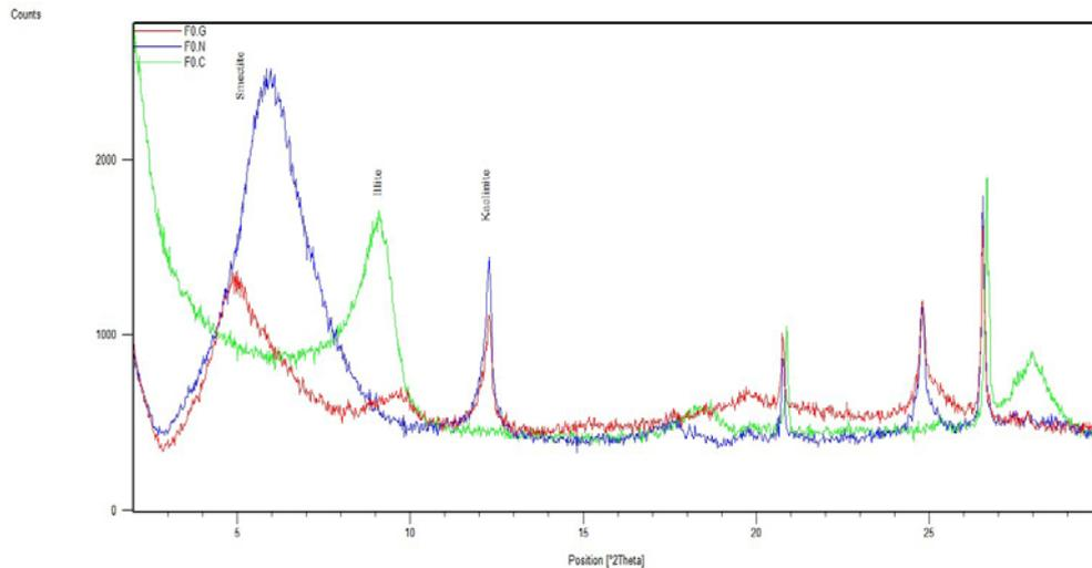
**Figure 2. XRD results for the undistributed sample.**
