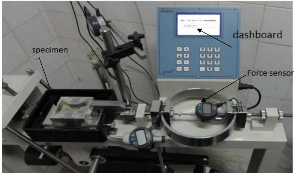
**Figure 6. Photo of direct tensile test used in this study**
