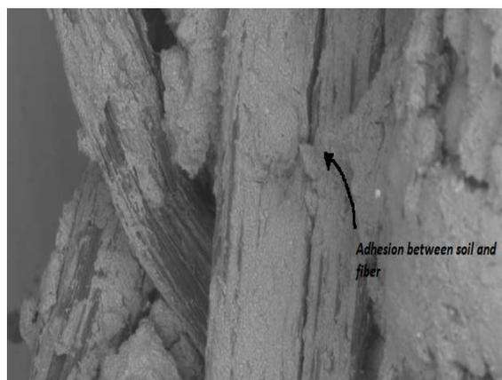
**Figure 5. MEB observation (x150) of the Alfa fiber embedded in the used soil: a good adhesion between soil and fibers.**
