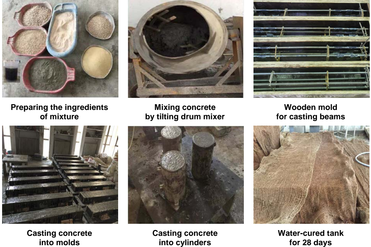
Figure 2. The mixing, casting, and curing of reinforced concrete beams.
