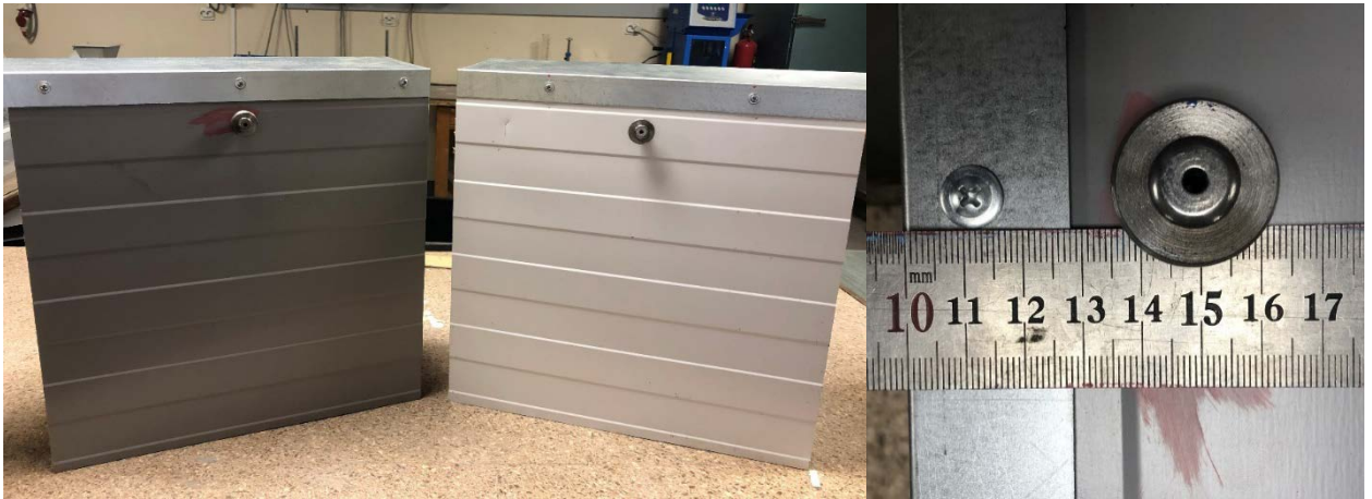
Figure 17. Coaxial and span fastening schemes.
