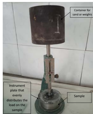
Figure 2. Device for determining the structural strength of an extruded layer of concrete mix.
